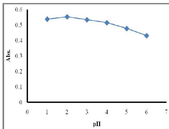
Fig 5. Effect of buffer pH on the reaction of LIS (15 mg/L) with HP CD.
