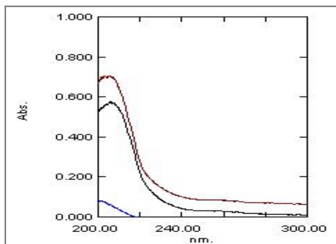
Fig 3. Absorption spectra of HP CD ( $3.0 \times 10^{-4}$   $\text{molL}^{-1}$ ) against water ( ), LIS (15 mg/L) against water ( ), and the reaction product of LIS (15 mg/L) with HP CD ( $3.0 \times 10^{-4}$  mol/l) against the reagent blank ( ).
